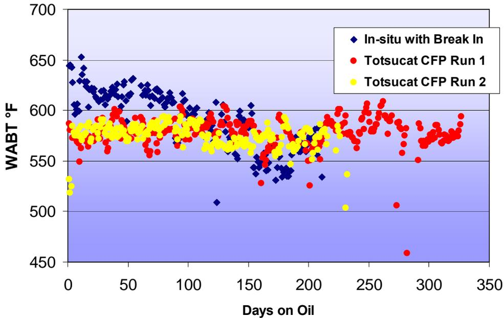
Figure 2 denotes the temperature difference across the reactor during each cycle. On average, Totsucat CFP provided a lower temperature gradient across the bed.
