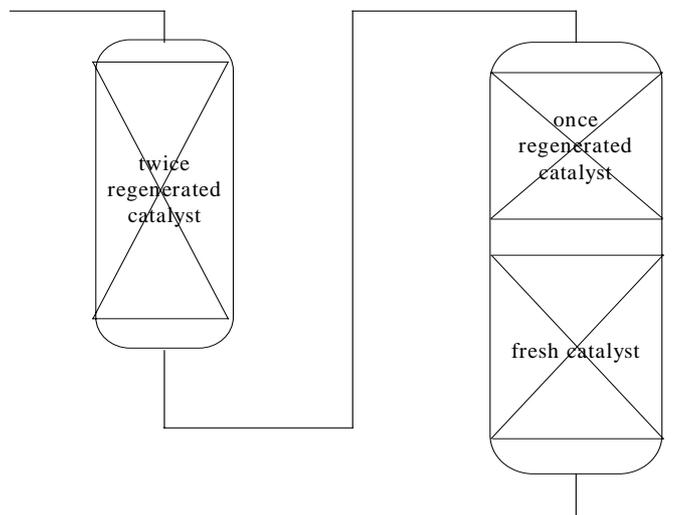
Protection of the HDS/HDN catalyst will be improved by using a demetallisation catalyst as top layer. These top layer demetallisation catalysts are usually not regenerable.
