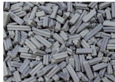
Guardian-CT is a CoMo Trilobe designed for use as bed grading in a variety of hydroprocessing unit applications. This shaped extrudate, typically loaded below other inert and active gradings such as Eurecat's Guardian-CR CoMo Rings, provides even flow distribution and pressure drop control along with moderate hydrogenation activity ahead of the main bed high activity HDS/HDN catalysts. Guardian-CT also offers excellent physical integrity.
