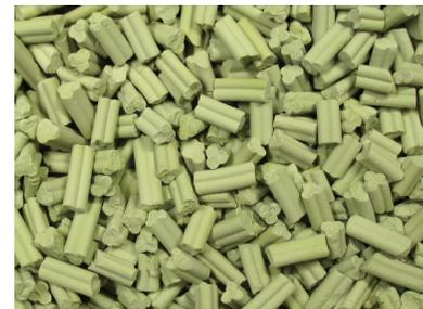
Guardian-NT is a NiMo Trilobe designed for use as bed grading in a variety of hydroprocessing unit applications. This shaped extrudate, typically loaded below other inert and active gradings such as Eurecat's Guardian-NR NiMo Rings, provides even flow distribution and pressure drop control along with moderate hydrogenation activity ahead of the main bed high activity HDS/HDN catalysts. Guardian-NT also offers excellent physical integrity.
